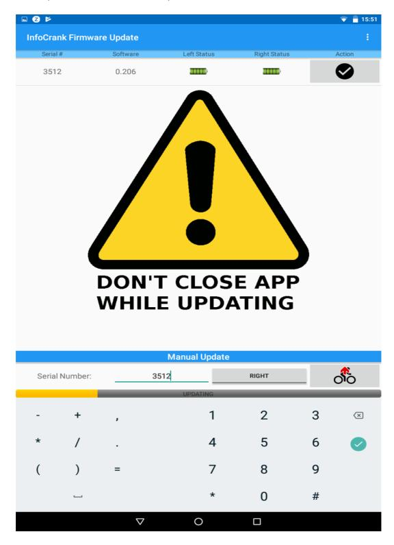
8. When the right crank is done, repeat the process on the left crank. The cranks are now restored with new firmware and you can revert to VINC and check the torque messages or just ride the bike.
