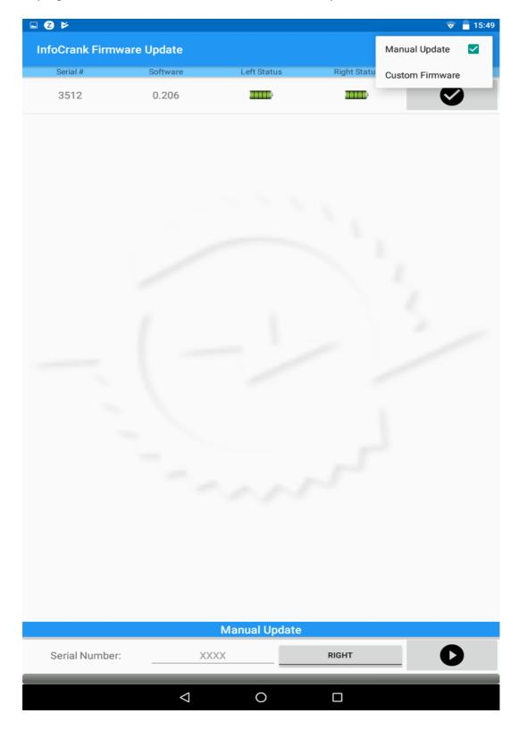
5. Type in last four digits of the serial number of crank and start with right crank. Press the start button.
