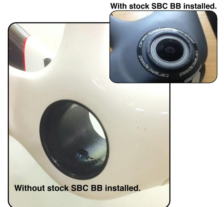
This is OSBB Road with Carbon Inner Shell. The frame measures 61.5mm Wide X 46mm Diameter.
